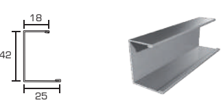
PROFILO | PROFILE "C" 18x42x25 L=4000mm
